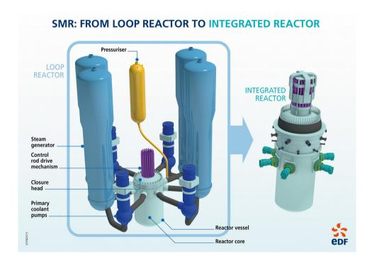
Compacting a full-scale nuclear reactor to obtain an integrated reactor design (source: EDF)
